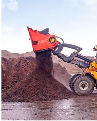
Figure 30. Screening bucket Source: ALLU
