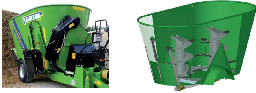
Figure 20. One shaft and two shaft mobile shredder (Source: Foresin )
